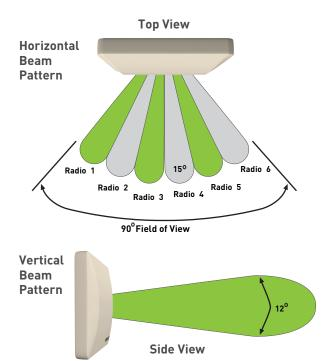
The Base Station constantly monitors the 6 radios for inbound client transmissions to determine the best path and then associates the client to a particular WLAN interface. This information is utilized by the Base Station to determine which WLAN interface to use to send traffic. To the client, the VT2210 Base Station appears as 6 individual WLANs. The client can roam across these WLANs just as it would roam across coverage cells provided by 6 separate APs in a typical WLAN environment.
